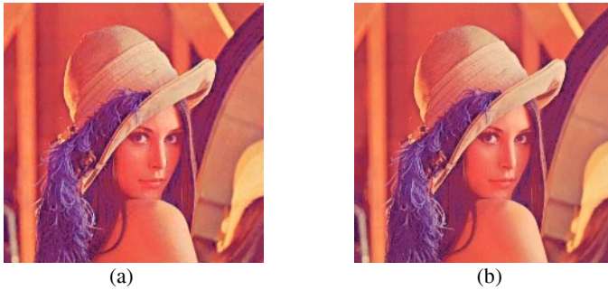
Fig. 6. The test image (512×512) and watermarked image. (a) "Lenna" test image. (b) Image embedded with a voice watermark ( \alpha_r = 0.035 , \alpha_b = 0.07 and PSNR = 40.12dB )
