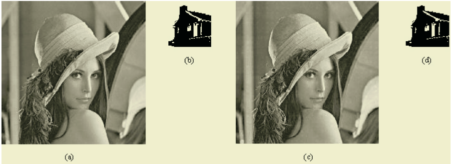
Fig. 5. Example of the Proposed Watermarking Approach. (a) Test Image Lena. (b) Watermark. (c) Watermarked Image (with PSNR = 40.24 dB). (d) Extracted Watermark with NC \approx 1.0.
